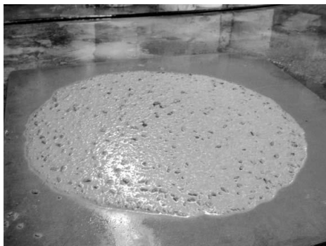
VSI = 2; Mortar halo, slight segregation
